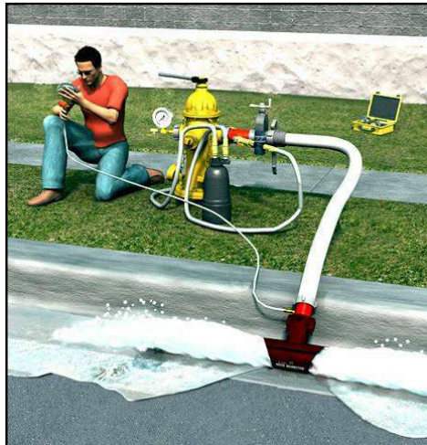
Hose Monster unidirectional flow testing, shown with optional de-chlorination system
